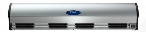
The EAQ-5T-H/EAQ-5TS-H series of Air Curtains feature internal structure made of SS304. Its outer frame is made from extruded anodized Aluminum Alloy. The impellers are directly driven. The motor used are of totally enclosed type with Class F insulation and self-lubricating ball bearings. It can also operate at 2 selectable speeds 'LO' and 'HI'.
